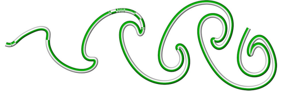
Figure 8. 2D cylinder data set. Visual comparison between the integrated streak line (green) and the ground truth (white). Their point-wise distance is plotted in Figure 9a, their Hausdorff distance in 9b (●).
