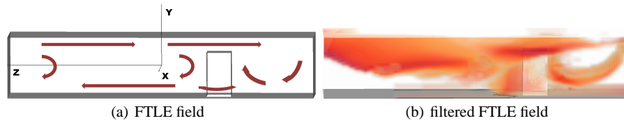
Fig. 5 (a) Schematic overview over the flow domain. (b) The FTLE field of a simulation of a bursting dam with parameters t_0 = 62 and T = 68 . The FTLE values greater than 0.25 are brushed (smooth lower bound 0.2). We see that we can identify expected structures around the obstacle. The upper rear part of the flow domain shows large regions with high FTLE values, possibly induced by shearing. (b) The FTLE filtered by sep(\mathbf{x}) < 0.45 (smooth lower bound 0.4).
