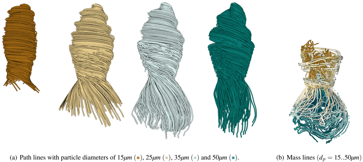
Figure 9: Hydrocyclones are used to separate particles in liquid suspensions based on density variations. As visible in Fig. 9(a), an increase of mass (and thereby inertia) causes particles to drift off the vortex core and to exit at different times. Mass lines in Fig. 9(b) expand and swirl around the bottleneck, which shows that lighter particles reside longer in the bottleneck.
