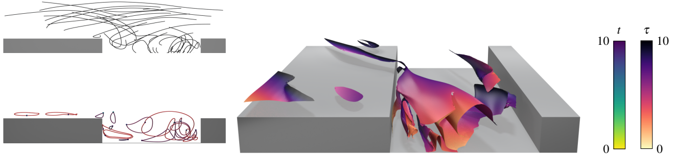
Fig. 6. CAVITY. Top left: Random path lines in the 2D cavity flow. Seeded particles move from right to left. Bottom left: Collection of recirculating path lines in and behind the cavity. The spheres mark the seed, color encodes integration time \tau (curves) and t (spheres). Right: Recirculation surfaces extended to in x - y - t -space. The surface color encodes the integration time \tau .
