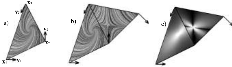
Figure 4.20: a) linear vector field inside the triangle \mathbf{x}_1, \mathbf{x}_2, \mathbf{x}_3 ; b) piecewise linear vector field consisting of two domain triangles; c) curvature plot of b) reveals that the tangent curves in b) are not curvature continuous.
