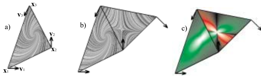
Figure A.18: (color version of figure 4.20): a) linear vector field inside the triangle \mathbf{x}_1, \mathbf{x}_2, \mathbf{x}_3 ; b) piecewise linear vector field consisting of two domain triangles; c) curvature plot of b) reveals that the tangent curves in b) are not curvature continuous.
