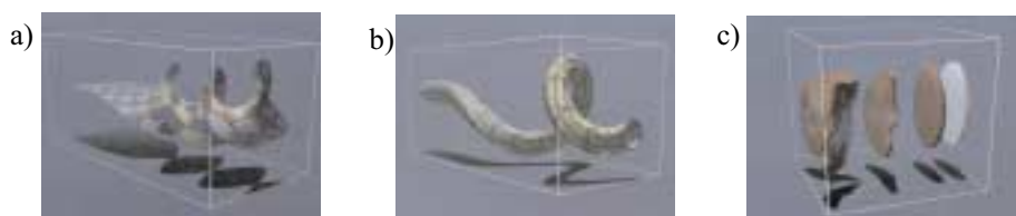
Figure A.22: (color version of figure 4.28): a) stream surface; b) stream tube; c) stream objects; (from [180]).
