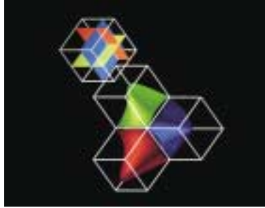
Figure A.3: (color version of figure 3.1): 2D slices for a point of interest in the volume; its three 2D scalar fields are visualized as height fields; the point of interest can be moved interactively (from [143]).
