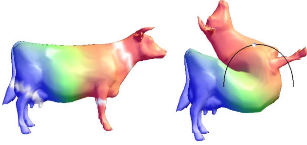
Figure 10. Due to the chosen boundaries (white), both the head and the front legs of the cow model undergo a full deformation.
