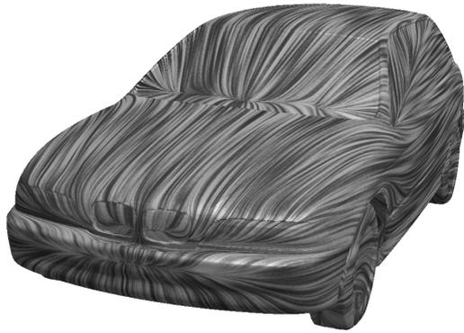
Figure 7: Texture-based flow visualization on a curved surface for an automotive CFD simulation.
