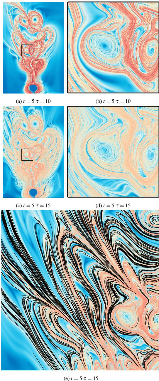
Fig. 4: BOUSSINESQ flow: FTLE field for different integration times with close-up views (a)–(d). Close-up with overlaid ridge geometry of the 1000 longest ridges (e)
